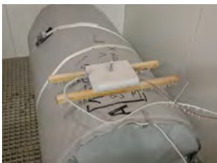
LIFERAFT STORED FOR 50HRS AT -70^{\circ}\text{C}
